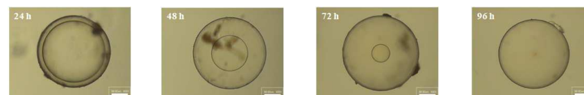
Figure 2. VMS photographs of s-PVA/P(VPi/VAc)/TiO 2 nanocomposite microspheres with skin/core structure by saponification time.
